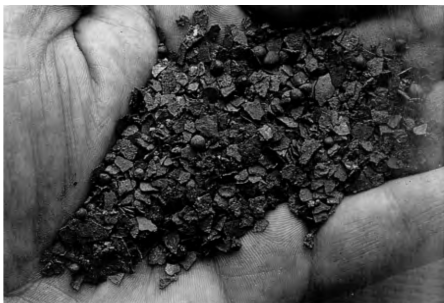
Hammerscale produced in the smithing of iron was a common find at Christ Church College. Both flake and spheroidal hammerscale are present. Flakes are fragments of the oxide/silicate skin dislodged by mechanical or thermal shock during forging and the spheres are small solidified droplets of slag expelled from within the iron during working.
